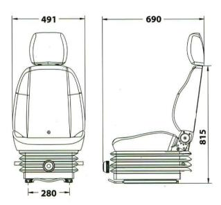
The KAB 525 is a mid back mechanical forklift seat. Like all seats within KAB Seating's product range, the KAB 525 incorporates user-friendly controls and an extensive range of ergonomic adjustments. These features ensure prolonged user comfort and therefore epitomise the KAB Seating slogan, "Enter The Comfort Zone".
